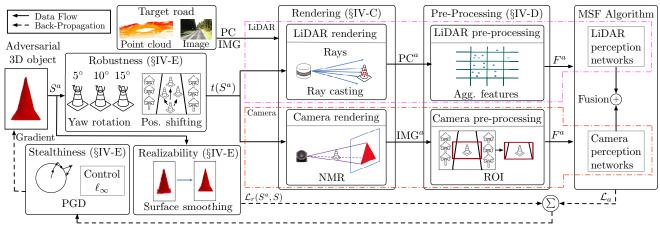
Figure 3: Overview of the optimization-based adversarial 3D object generation in MSF-ADV.
