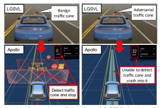
Figure 11: Screenshots of Apollo and LGSVL in the end-toend attack evaluation with benign and adversarial traffic cones. Across 100 runs, the crash rate is 100% for adversarial case, and 0% for benign case.
